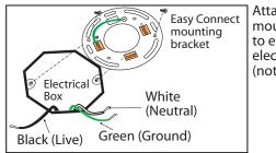
Attach easy connect mounting bracket to electrical box with electrical box screws (not included).
